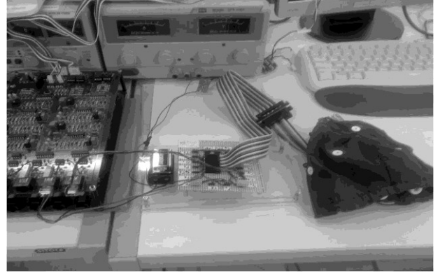
Fig.1 EEG device developed by the team connected to electrode cap
