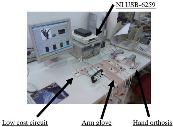
**Figure 5. Experiment Setup**
