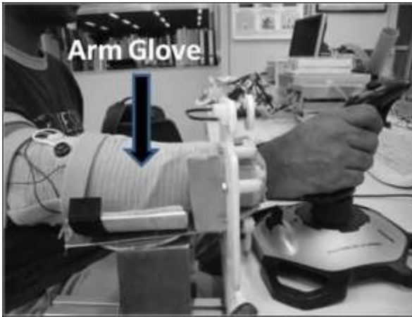
Figure 1. Table top set up of arm glove with joystick
