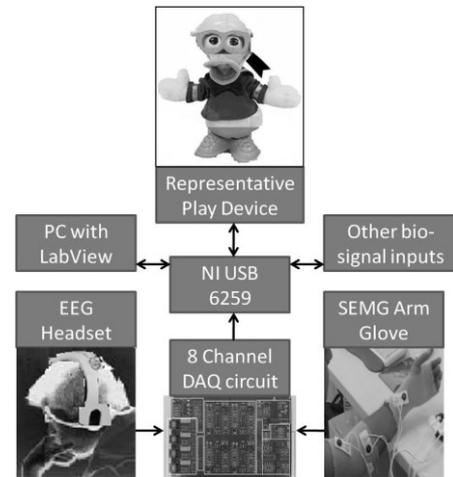
Fig.1. Schematic of the development platform
