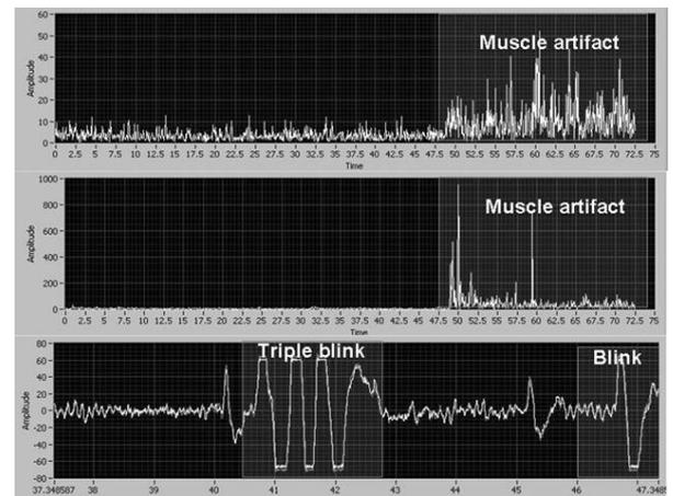
Fig. 8. top – gamma wave of eyes squeezing artifact with eyes closed; middle – gamma wave of frowning artifacts in eyes open condition; bottom – blink and triple blink detected as saturated signal
