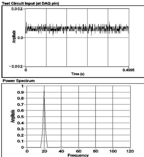
Fig. 6: Power spectrum of test output for circuit operating in EEG Mode. The noisy input signal is shown above.
