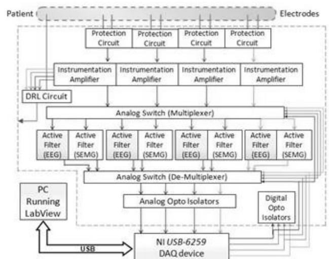
Fig.2. Layout of the 4 channel SEMG/EEG data acquisition system. 2 such modules are used to make up the 8-channel DAQ circuit described in Fig.1
