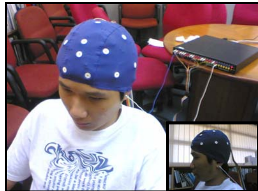
Figure 4: Pilot experiment setup on the test subject using Mindset 24R
